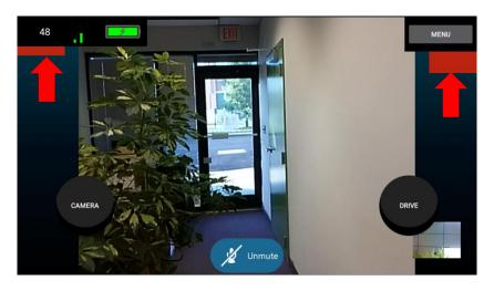
Note: To reduce the likelihood of a high speed collision (e.g. driving the MantaroBot into a wall) a feature has been included in the MantaroBot that reduces the robot's forward speed when it detects an obstacle 30 cm ahead of it. Note forward speed is not reduced if the robot is moving slowly. A red area will appear on the pad to indicate that the speed has been limited. These sensors will not detect all types of wall surfaces or prevent the MantaroBot from falling down steps or stairs.
